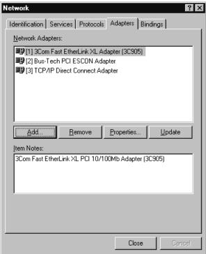
Figure 5-17. Network Adapter List with TCP/IP Direct Connect
